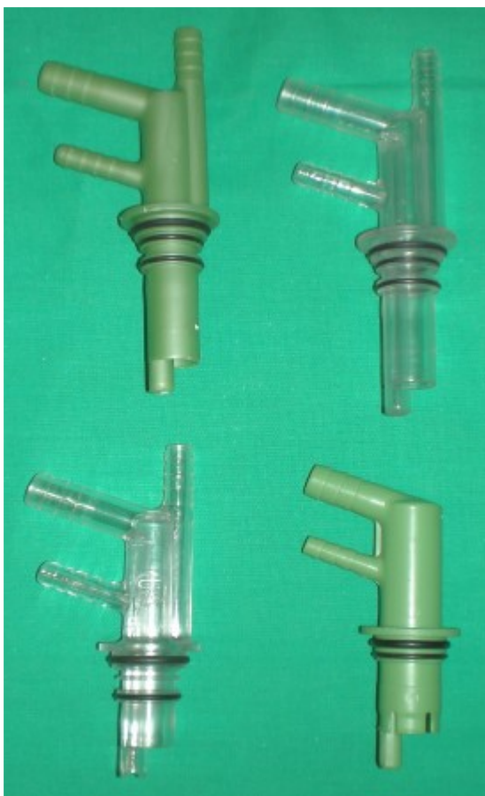
Nozzle for formation with acid recirculation
